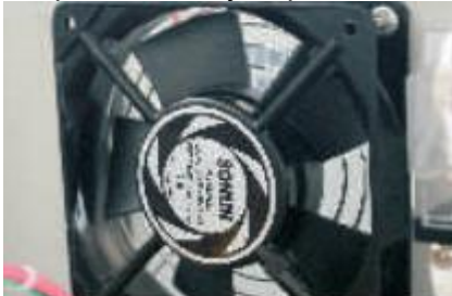
Fan: Long life of 100,000 hours automatically start working when the system temperature reaches a certain temperature.
